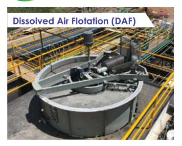
In The DAF unit suspended solid, Fat, Emulsified & Free Oils are removed from effluent. Here chemical are dosed from dosing tanks. Air Compressor and HPP are provided for this system.
