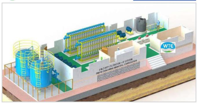
Ultra Filtration is a membrane based technology which is used for removal of suspended particles up to 0.01 micron size which results in SDI reduction. These membranes are available in 10 Kilo Daltons & 100 Kilo Daltons molecular weight cut off configuration as per the process requirements.
