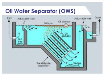
Oil water separator is technology which remove free oil from water till <5ppm with the use of API / TPI, oil skimmer and coalesce column
